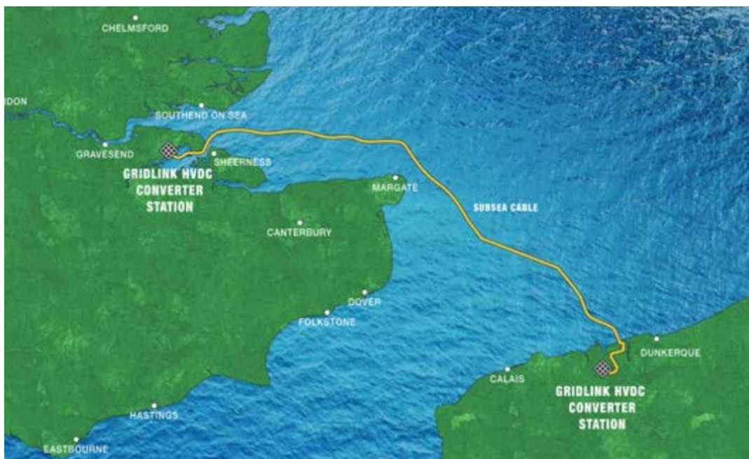
Figure 4 – GridLink cable route and converter station sites
